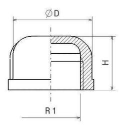
**Norms:** Male thread according to EN10226-1 Female thread according to ISO 228-1
